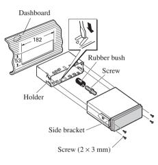
• After installing the unit into the dashboard, reattach the frame.
